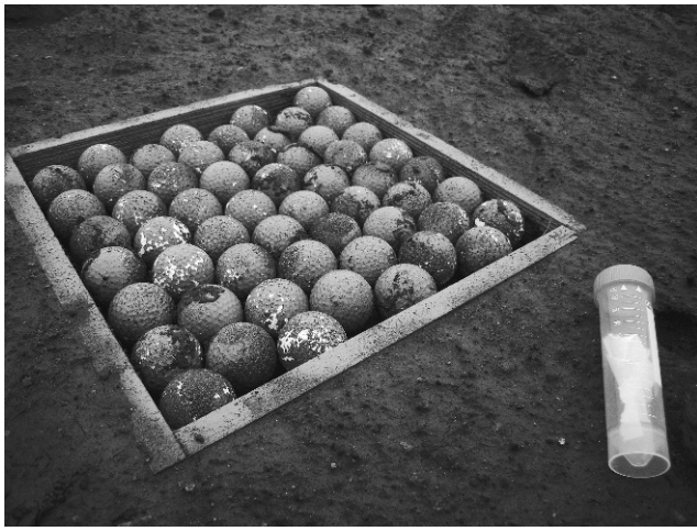
FIGURE 2. Aerial plankton/arthropod biomass fallout collectors built to specifications of Edwards (1986) and Edwards and Sugg (2005).
