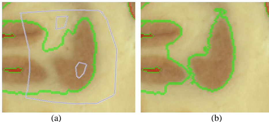
Figure 22: Sample boundary competition with user-selected mean colors for a white and gray matter boundary (a_vm1070.png). (a) The required user inputs: The outermost blue loop defines/limits the area in which competition will take place. The smaller loops indicate the sub-regions selected to represent the colors for the two tissues. (b) The result of the competition. Notice the improved boundaries in the competition area and the unchanged boundaries outside of it.
