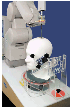
Figure 1: The IEEE standard SAM phantom that is currently used to certify compliance of cell phones with relevant safety standards [2].
